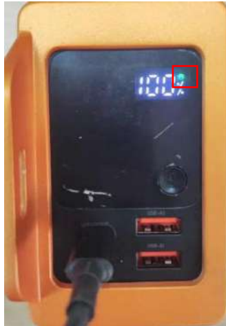
Figure 2-3 T10 system battery turn on diagram
