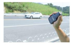
With laser measurement, surveyors can collect the coordinate of points that they cannot reach directly or in dangerous places, like the high voltage towers, manhole covers on busy roads, ensuring the safety of personnel.
