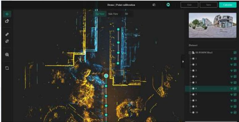
2. For projects with height difference errors. It can also be adjusted by point calibration, the viewpoint is switched to **side view**, and the height of the points can also be calibrated by disconnecting the connecting line.
