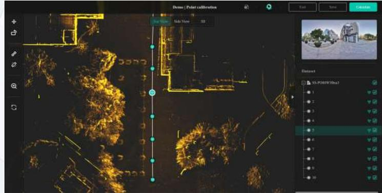
2. Select the Disconnect tool to disconnect the part to be adjusted from the rest and select the part to be adjusted. The selected part is highlighted in yellow. The panoramas of the selected point and the point number are displayed on the right side of the point column.
