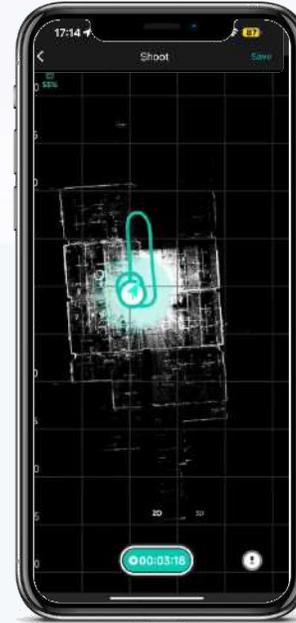
7. When adding scan points in SLAM scanning, the scan page will display the point number, you can click the point to preview. The maximum number of points in a SLAM scan project is 500, and the distance between points is not limited.
