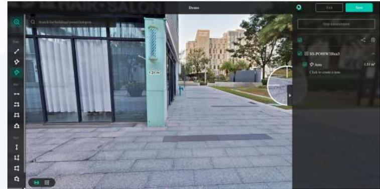
3. Switch to another point to see if the measurement point is aligned, if there is no alignment, you can drag the measurement point to the correct position by selecting it.
