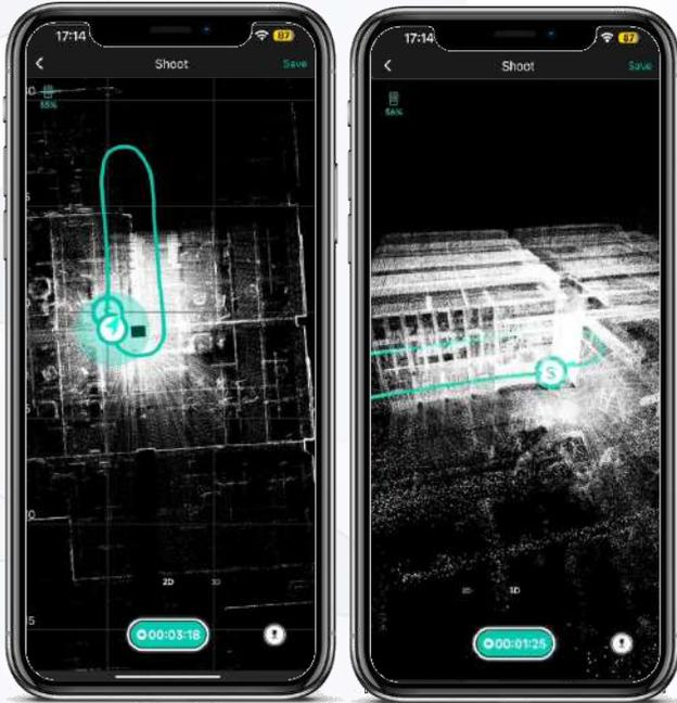
5. During SLAM scanning, you can use the 2D or 3D button to change the view to preview the real-time point cloud data.
