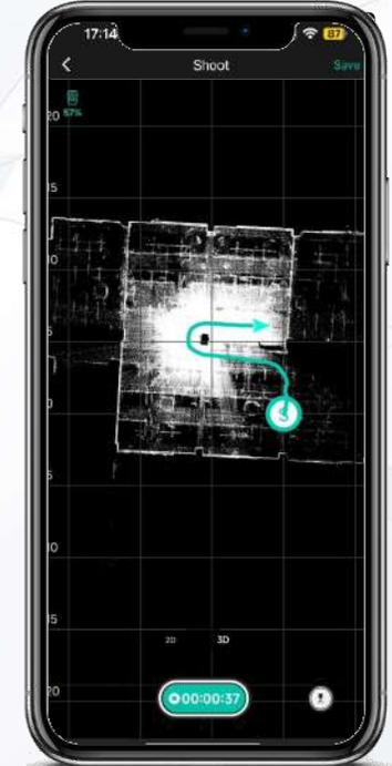
4. Move to capture the point cloud data, the scanner should move smoothly and at a steady speed, and the camera lens should always face forward and along the moving direction. The APP will display the moving track and point cloud data in real time.
