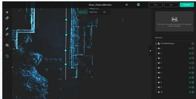
4. For points with GNSS data, you need to turn off the **GNSS data**
