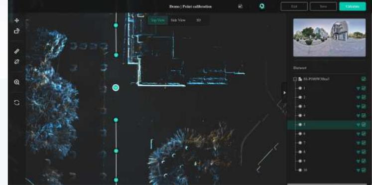
3. Calibrate the adjustment part by rotating and moving. During calibration, you can change different views to determine the effect of the adjustment.
